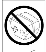
Regularly check that the muffler is securely attached to the chain saw.
